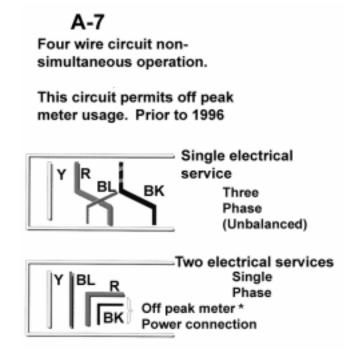
\*Some electrical utilities give discounts if electricity is used during "Off Peak" times of the day. This circuit allows use of an "Off Peak" meter, which interrupts power to the lower element during the time of day when electricity is more expensive. This customer relies on additional hot water storage to meet their needs while this element is off.
